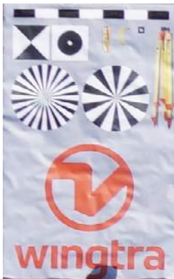
Sony RX1R II 42 MP camera (with a WingtraOne drone) GSD: 0.7 cm (0.3 in) / px
