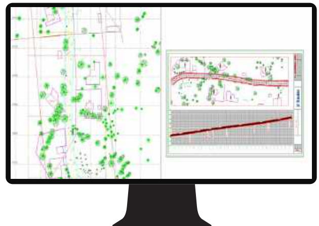
Draft plan and profile sheets with dynaviews
