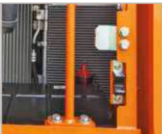
Battery cut-off switch
