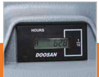
Hour meter (from ground level)
