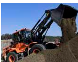
Cinematica parallela (Tool Carrier)
