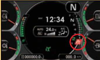
AdBlue® level gauge and refill guidance
