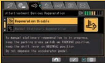
Aftertreatment device regeneration screen for the KDPF
