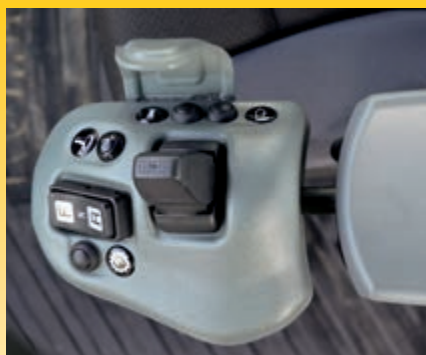
Komatsu short lever steering (K-SLS) (option)
