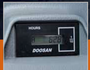
Hour meter (from ground level)
