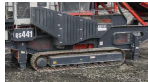
Four jacking legs for increased servicing capabilities
