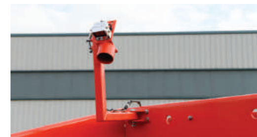
Camera and level sensor to ensure continuous feed
