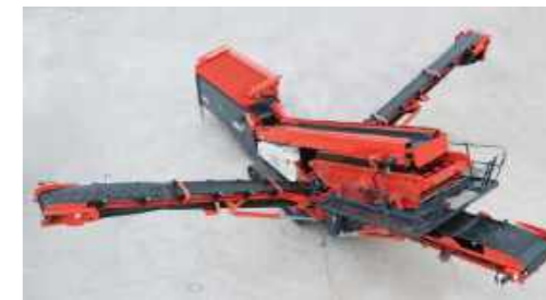
Three discharge conveyors
