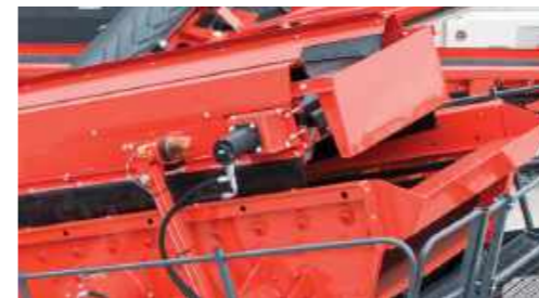
Hydraulically retractable main conveyor
