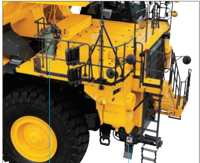
Grease pump pump and reservoir Refill port
