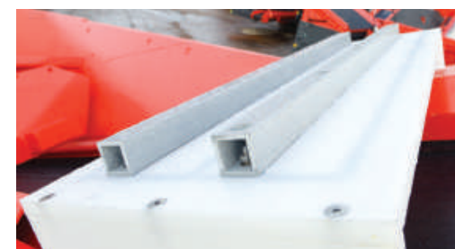
Bridge coil metal detector for controlled detection
