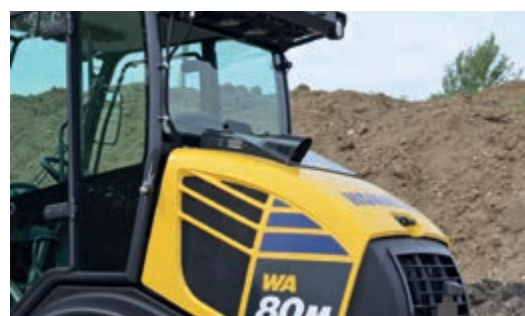
Standard heated rear window and a newly designed, low-profile exhaust pipe ensure improved rear visibility (to ISO 5006).
