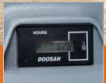
Hour meter (from ground level)
