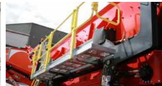
Hydraulically folding maintenance platforms
