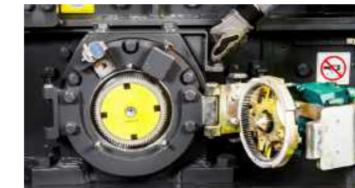
Patented rotor locking and positioning device for increased safety
