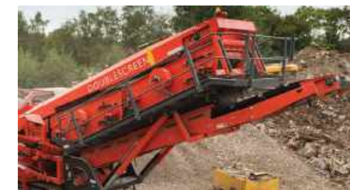
Hydraulically folding walkways for ease of maintenance
